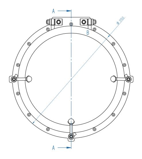
MADE IN STAINLESS STEEL AISI 316 L FINISHING MIRROR POLISHED PLATE DIMENSION ACCORDING CLASS OPTION FIXED TYPE OTHER DIMENSIONS ON DEMAND
