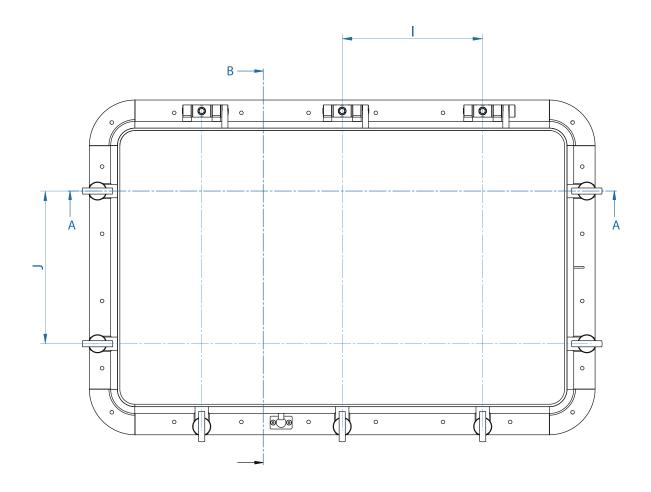
MADE IN STAINLESS STEEL AISI 316 L FINISHING MIRROR POLISHED PLATE DIMENSION ACCORDING CLASS OPTION FIXED TYPE OTHER DIMENSIONS ON DEMAND
