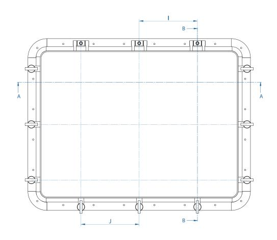
MADE IN STAINLESS STEEL AISI 316 L FINISHING MIRROR POLISHED PLATE DIMENSION ACCORDING CLASS OPTION FIXED TYPE OTHER DIMENSIONS ON DEMAND
