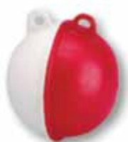
43395 Surface Float w/2 Eyelets, Spherical, white-red Overall Height: 15cm, Ø 13cm, top eye 1,2cm, weight: 130gr Buoyancy: Overall 542gr, In use 271gr
