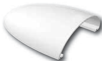
54386 Ventilation Clam Shell Cover For additional protection against heavy water intrusions. Suitable for 3" and 4" ventilators. To be fixed on top of the ventilator with 3 nylon fasteners. Made from polyamid, shock and UV-resistant. Compatible with common sealants and impervious to acetic acids. (215x180x70 mm)
